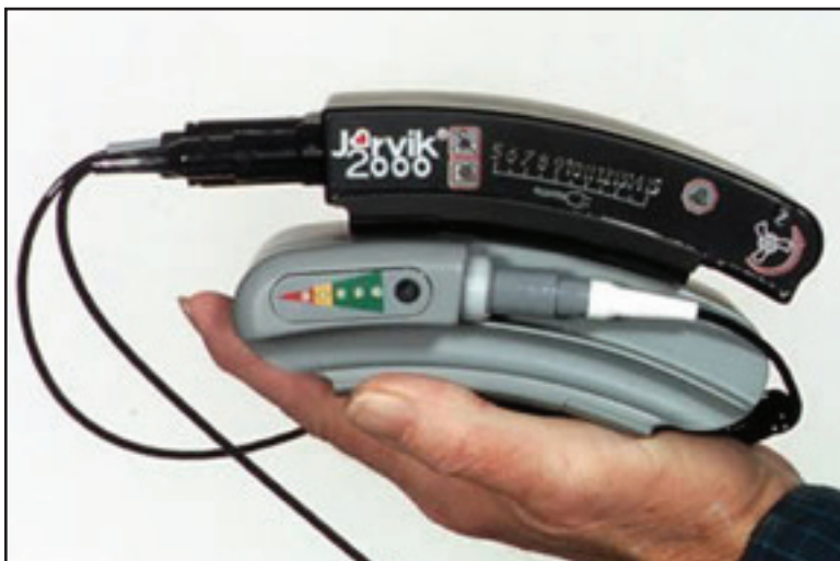
Controller attached to the portable Li-ion battery.
