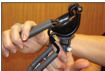
Release purge valve.
